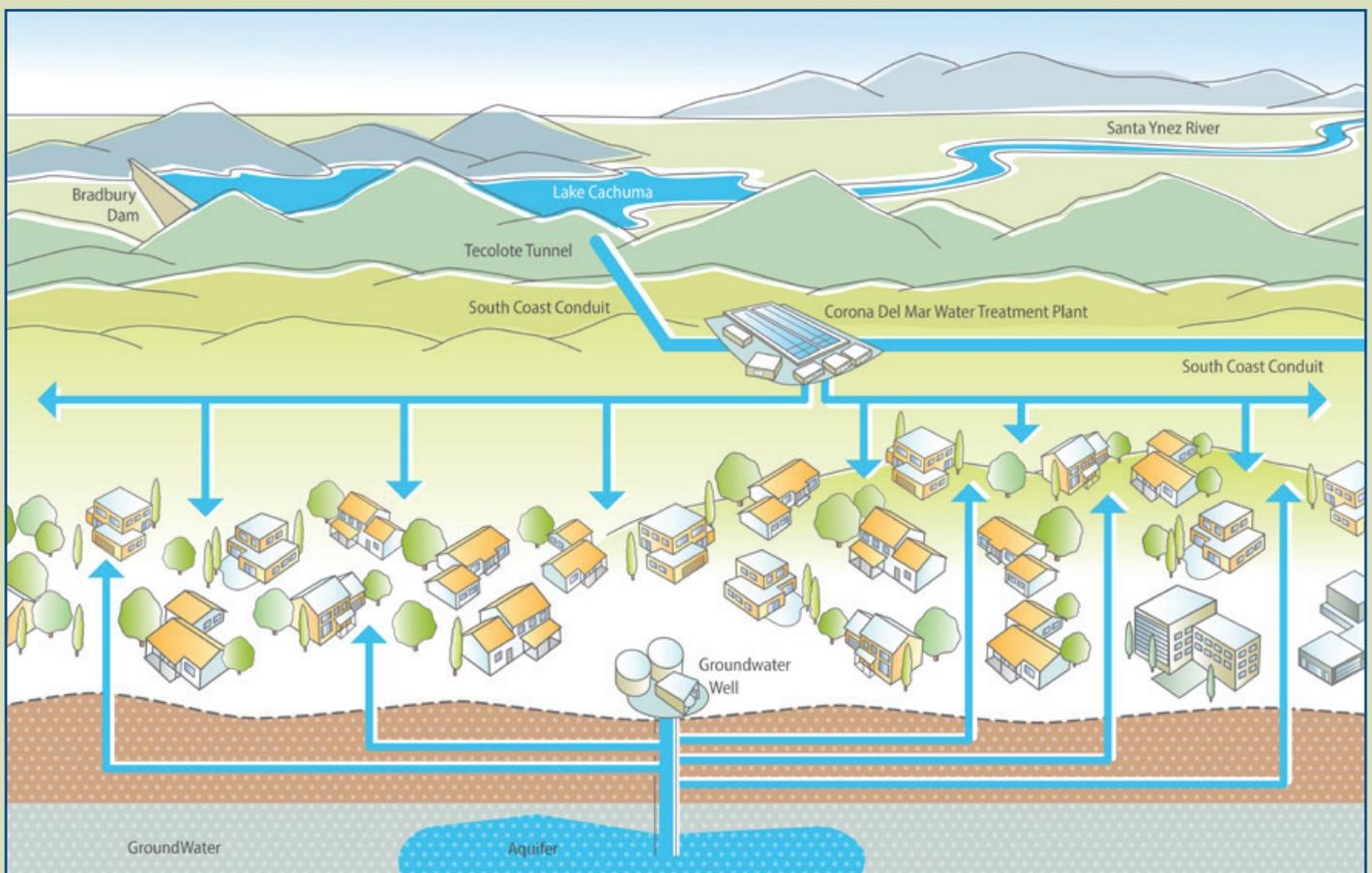
Unlike water from Lake Cachuma, which flows downhill through a gravity-fed system, groundwater must be pumped through 19 pressure zones within the District distribution system, and even uphill to many customers. Operations and maintenance costs associated with pumping and delivering this diverse water supply mix are higher, but the result is improved reliability and resiliency that has led to greater emergency preparedness.
